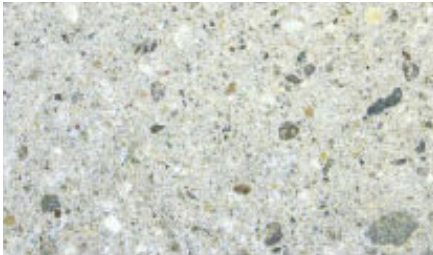
CONCRETE KNEE-WALL LIGHT SANDBLAST WITH GRAY LIMESTONE COLOR
